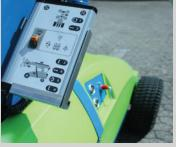
Wired remote control allows accurate placement of materials
