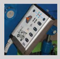
Multifunction control panel in operator friendly design with integrated buttons. Signal lights and double action safety keys are both in the standard setup on the Winlet 350TH.
