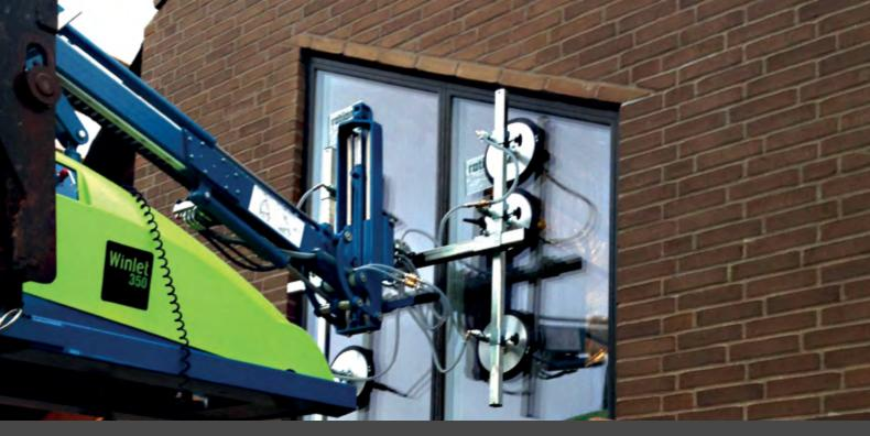
The Winlet 350TH has a hydraulic system which makes it independent from the telehandler
